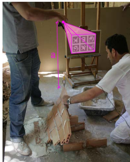
Figure 2. Implementation of the system, with a webcam, a marker board upright and the use of a dead load to precisely locate the reference point.
